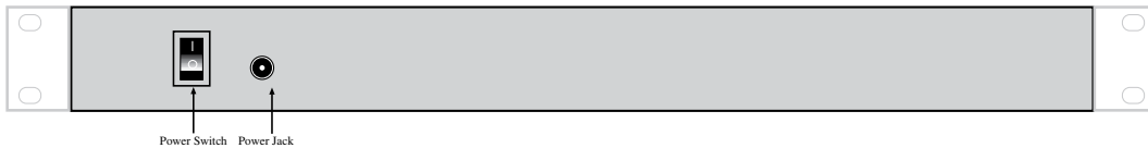
Figure 2: Rear Panel of the IMS 1000
